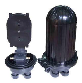
The FOC-10 Fiber Closure can be used for mid-span and is often the primary interface between the outside plant cable and distribution equipment or indoor cable. It accommodates up to 80 single fusion splices in a low weight, compact design, the versatile and reliable design lends itself to multiple mounting options and deployment environments.
